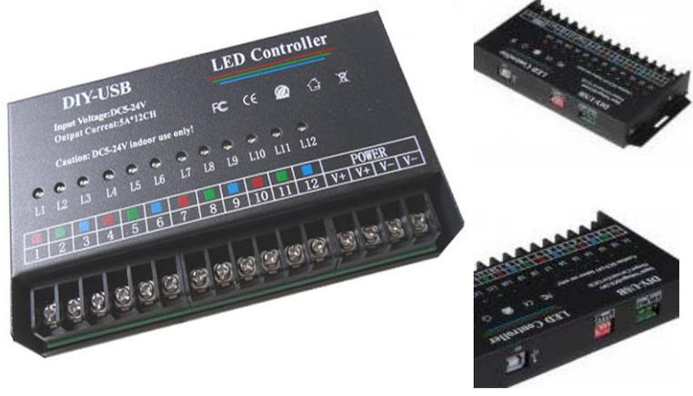
1. a single monochrome controller can control 12 channel signal color or 4 group RGB sourcing
