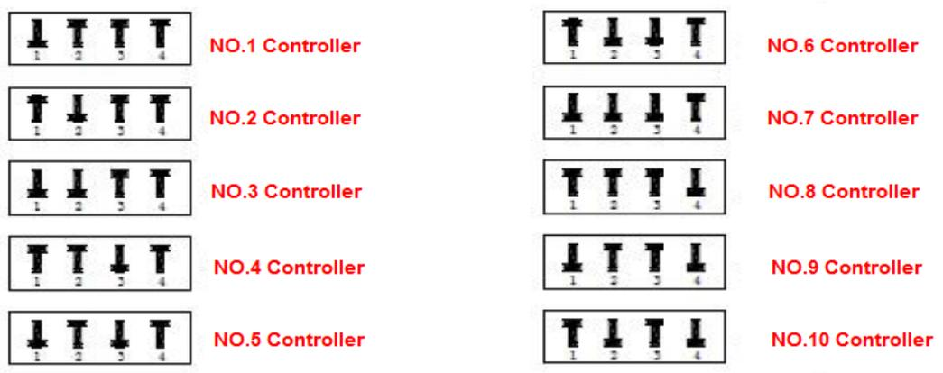
Please Dial the DIP switch for set controller serial number. When finish edit scenes, we need download all scenes to each controller, The controller can Identify their controllable channel base on their serial number
