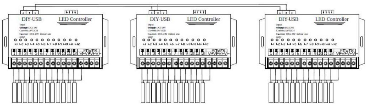
Max 10 Pcs controllers synchronous cascade, First controller' A and C Port connect with other 9pcs controller' A and B port as above drawing. Max cascade distance is 50meter for any two controllers
